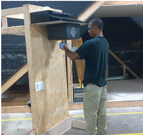
Jeremy Morris at WARM Training Center, Detroit, adapts Energy Conservatory's Exhaust Fan Flow Meter (the black box) to measure range hood flow. (Steve Christensen)
