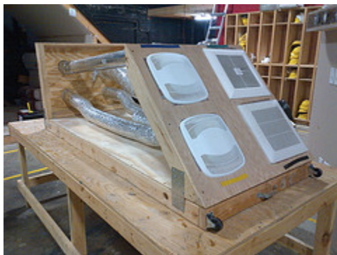
This prop, assembled by DOE-Funded WARM Training Center in Detroit, gives hands-on access to practitioners (auditors and contractors) to help select appropriate equipment for whole-house ventilation, as well as to overcome spot deficits. (Steve Christensen)
